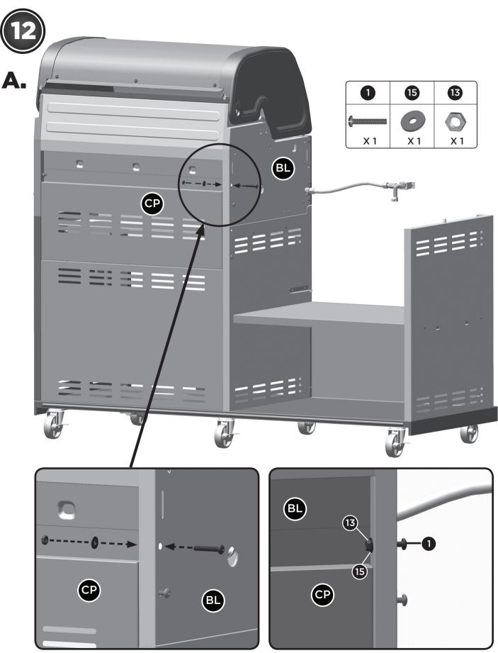
Anchor screw: Only tighten screw halfway, as shown.
